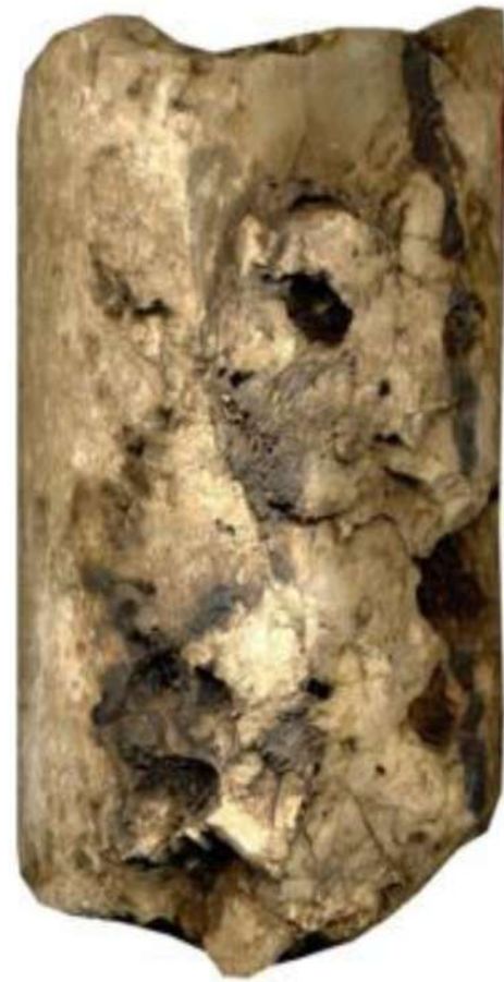
Figure 4—Brecchia core from the upper Cretaceous, showing vugular porosity. After Ref. 40
